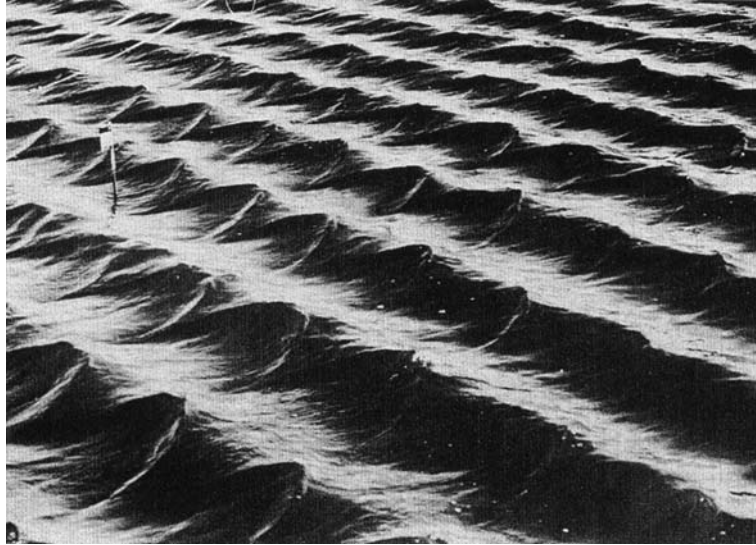
Fig. 4.13. Three-dimensional wave configuration resulting from oblique Type II instability, for s = 0.33 (from Su, 1982).
