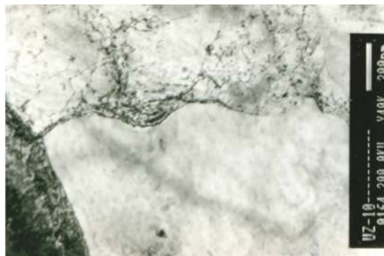
Figure 9. TEM micrograph of dislocations accumulating on the rows of precipitations.
