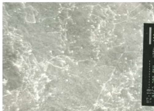
Figure 8. TEM micrograph of the interaction between precipitates and dislocations [20].
