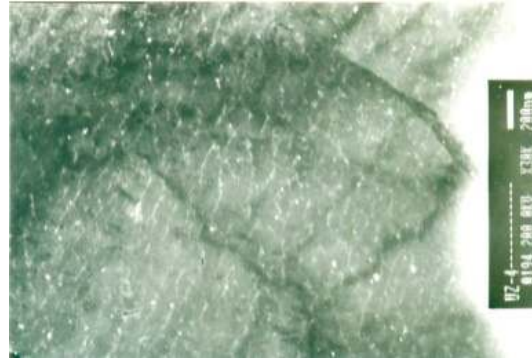
Figure 5. TEM micrograph showing the onset of strain-induced precipitation at 963 °C, low temperature (LT) variant.
