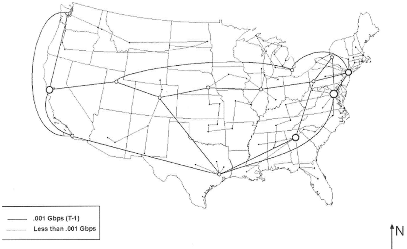
FIG. 2. NSFNet backbone and regional research networks, 1989. Compiled from individual maps in Quarterman (1989) and Salus (1995). Gbps, gigabits per second.
