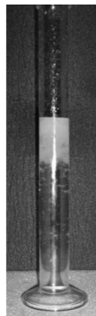
Fig. 3. Ice granules mixed with ESTISOL™ 240/COASOL™ at -25^{\circ}\text{C} .
