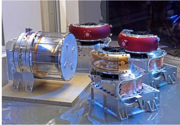
Fig. 4 Photograph of flight JADE-I ( left ) and JADE-Es ( right ) in the clean room, just prior to spacecraft delivery. Two of the JADE-Es ( rear ) have their protective “red-tag” covers on, while one ( front right ) and JADE-I have theirs off to show the open, gridded apertures
