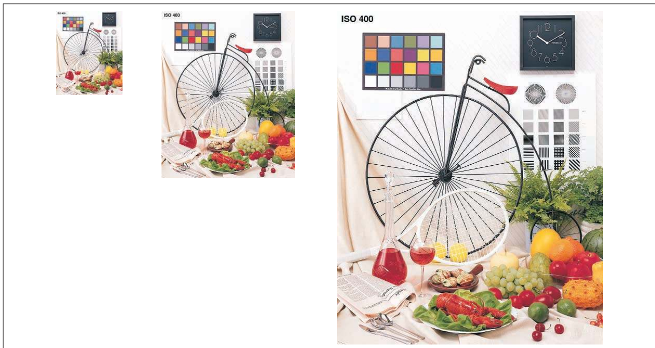
▲ 18. Example of the progressive-by-resolution decoding for the color image “bike.”
