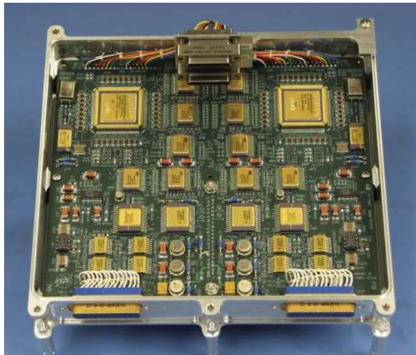
Fig. 22 Fluxgate magnetometer digital card in its frame prior to assembly. The digital system is dual hardware redundant (note symmetry) and only one side is powered at a time; the other is cold spared
