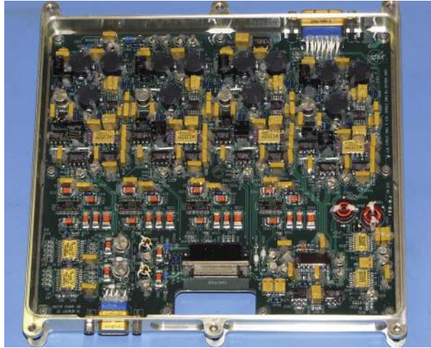
Fig. 19 One of two analog and A/D cards in its frame prior to integration. The card is designed to occupy either of the two analog positions so that both may be spared with an identical card
