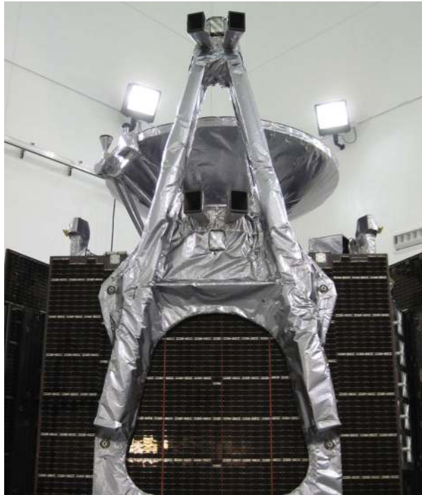
Fig. 24 Juno spacecraft in launch (stowed) configuration at Lockheed Martin's Watertown facility during environmental testing. The magnetometer boom, and magnetometer sensor suites (camera head light baffles prominently displayed) are wrapped in thermal blanketing
