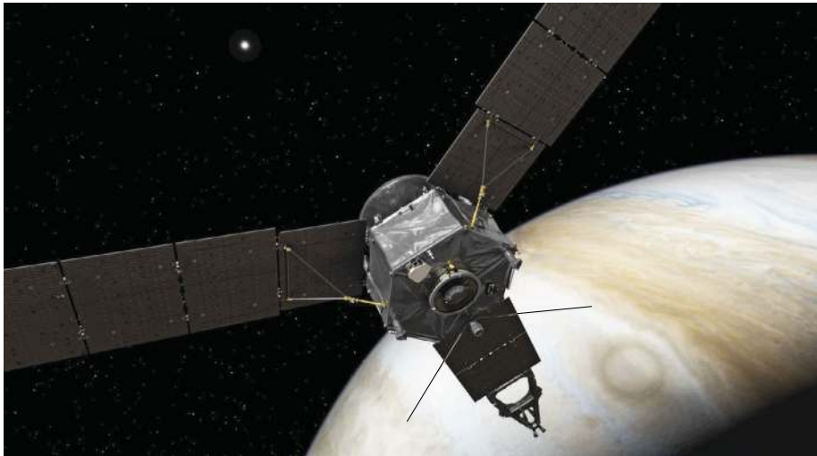
Fig. 15 Juno with Waves electric antenna deployed from the aft flight deck. The sensitive axis is perpendicular to the solar panel containing the magnetometer boom (spacecraft x axis) and the spin ( z ) axis
