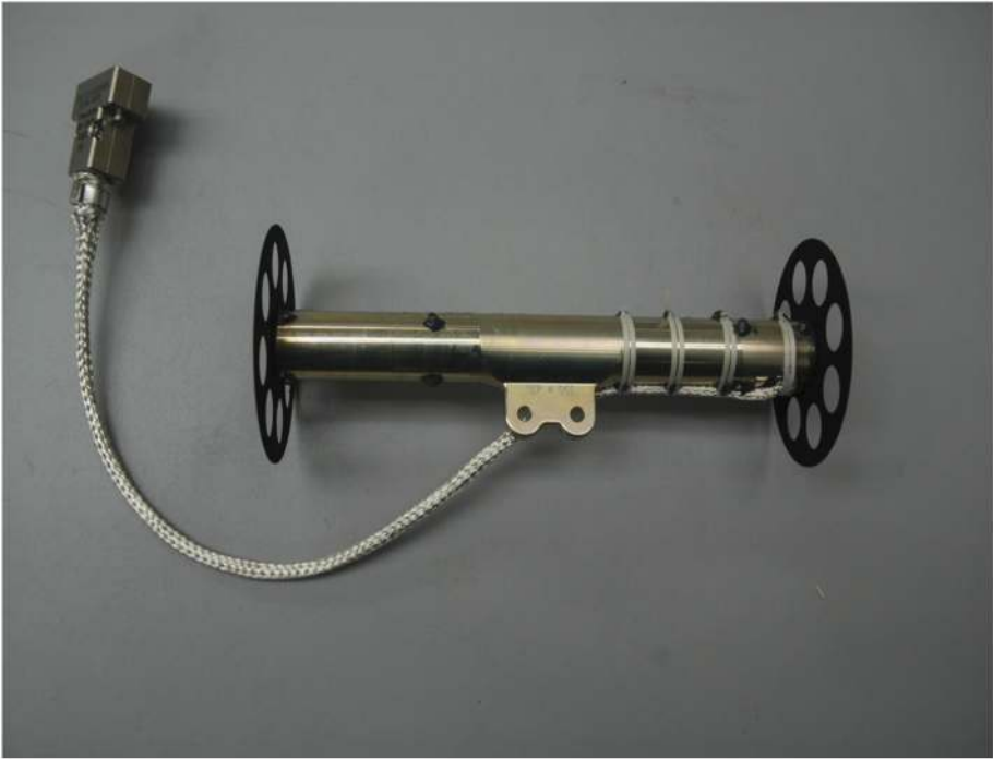
Fig. 16 This is a photo of the Juno Waves search coil antenna. The ‘wheels’ at the ends are standoffs designed to support the antenna’s thermal blanket. The search coil is body-mounted to Juno with its long (sensitive axis) parallel to the spacecraft spin (z) axis
