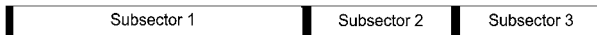
Fig. 27 Structure of the rotational (and timing) subsectors in the JEDI data accumulation scheme that allows us to sub-commutate in a flexible manner between the 3 different species collection modes: electron spectra, ion spectra, and ion species. One can choose to use a cyclic of combination of modes within these subsectors. There are 60 sectors per spin, and so this pattern of subsectors occurs 60 times per spin
