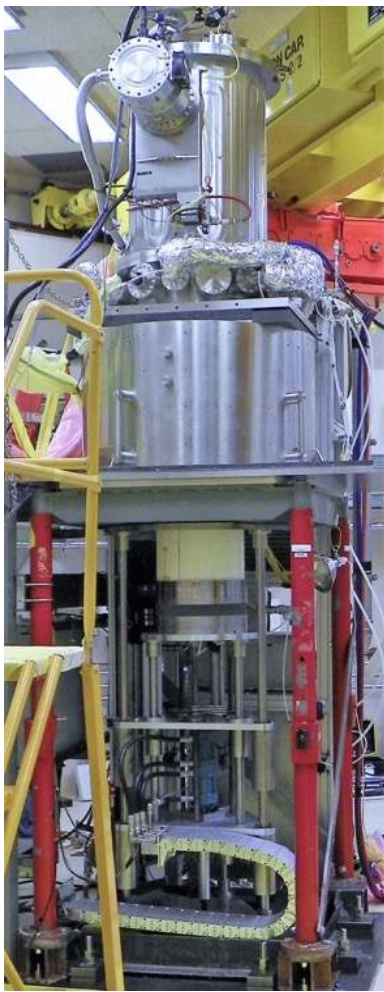
Fig. 5 Completed KRUSTY experiment setup with Comet machine, facility shielding, and vacuum system with enclosed power system and core
