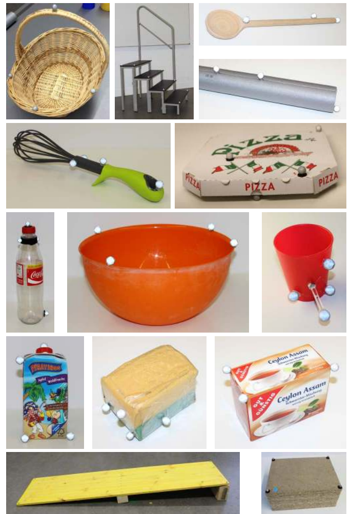
Fig. 6: Exemplary environmental elements and objects with markers attached to them for simultaneous capturing of subject and object motion.
