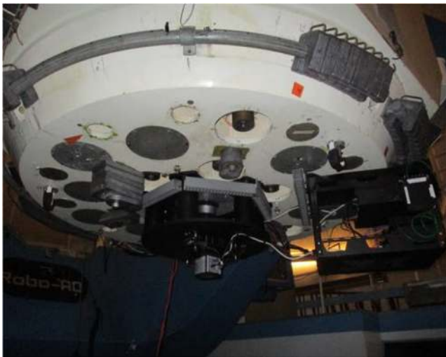
Figure 3. Photograph of KPED and electronics rack installation.
