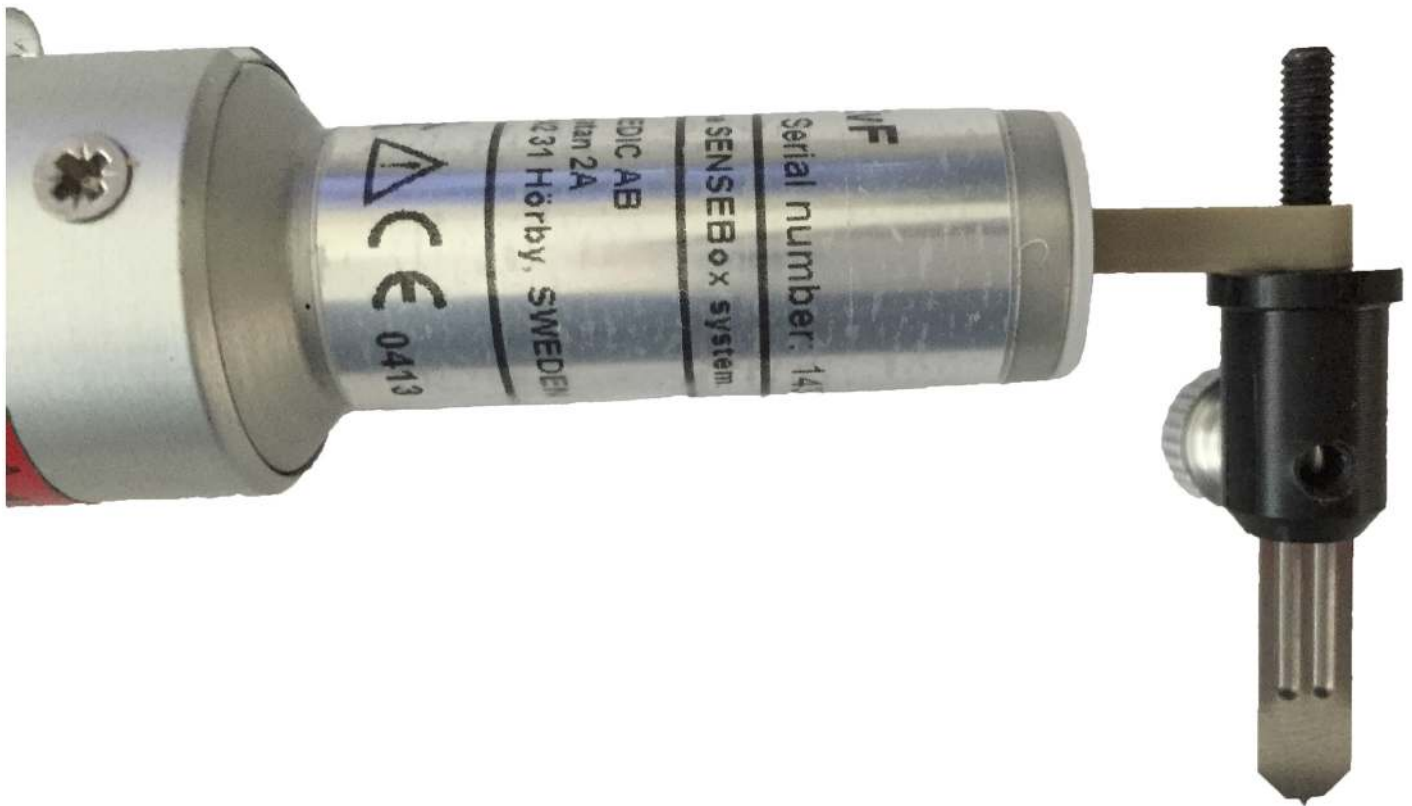
Fig 1. The setup of the SPT lancet attached to the SENSEBox Electronic von Frey weight transducer.
