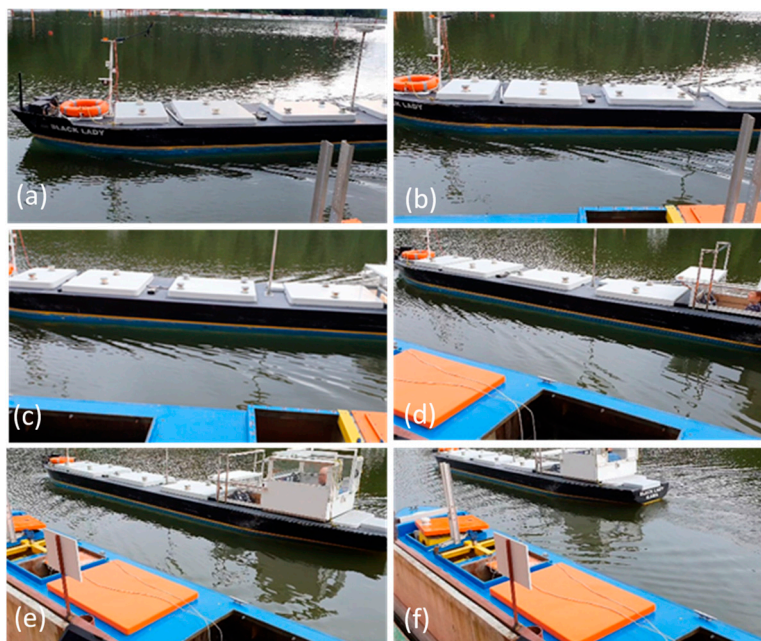
Figure 11. Wave system generated by the passing ship model s = 2 , Fn = 0.155 : (a) l = -0.5 ; (b) l = -0.25 ; (c) l = 0 ; (d) l = 0.5 ; (e) l = 0.25 ; (f) l = 0.75 .
