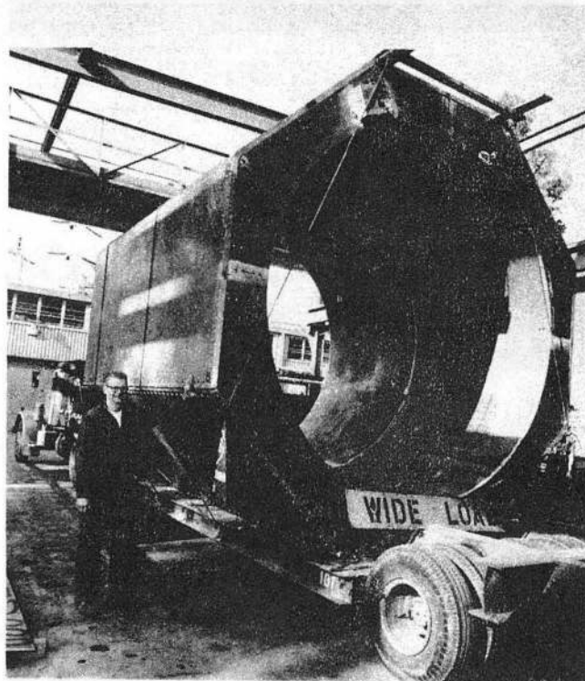
Fig. 1. Octagonal "Squirrel Cage" which provides a vacuum jacket for eight barrel modules as well as their mechanical support.
