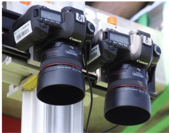
Figure 1 Stereo rig. Two cameras are fixed with a profile system and slightly turned to each other to capture the same scene. A remote-control release allows for synchronous triggering. In this setup the baseline was adjusted to b \approx 200 mm.
