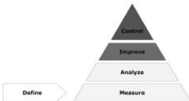
Fig. 2 - the DMAIC Algorithm used in LSS Project.
