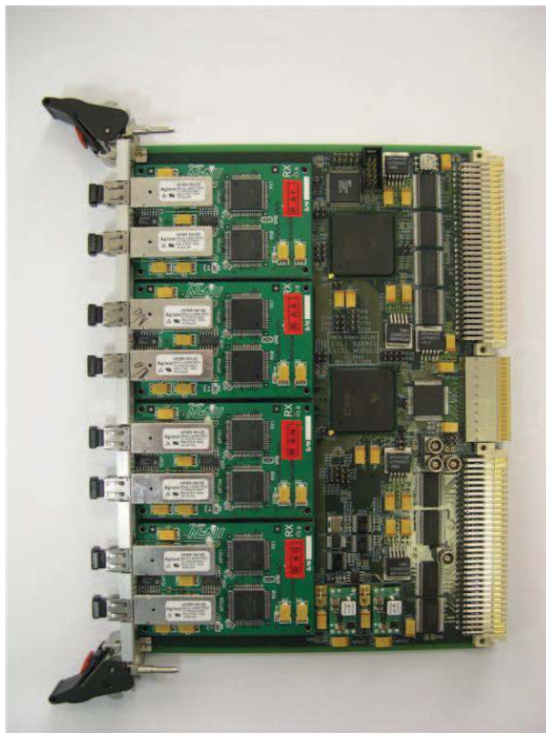
Figure 18. Photograph of a Sector Logic (SL) board. The four RX optical link mezzanines are mounted on the left, while the VME FPGA is on the upper right side. In a central position, the SL data processing element can be seen, while the serializer shipping data to the ROD is very close to the central backplane connector
