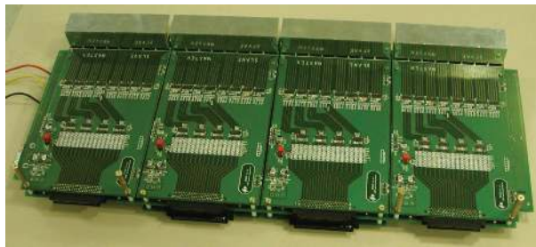
Figure 8. Picture of a Splitter circuit, as seen from the \eta side, out of its encasing
