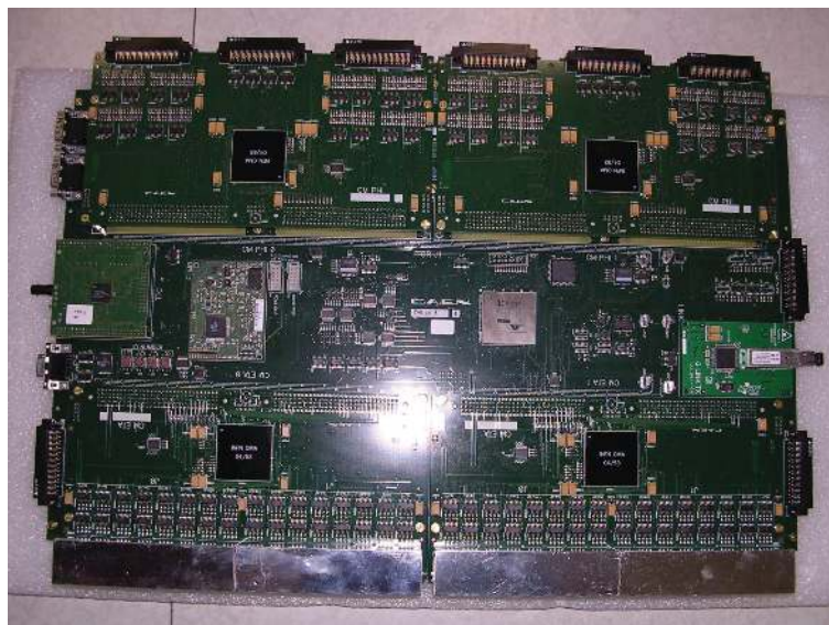
Figure 14. picture of a PAD out of its encasing. On the lower part the two \eta CMs add-on boards can be seen. In the central part, starting from left: TTCRQ, ELMB, PAD FPGA, Optical link mezzanines can be seen. In the lower part the two \phi CMs add-on boards can be seen
