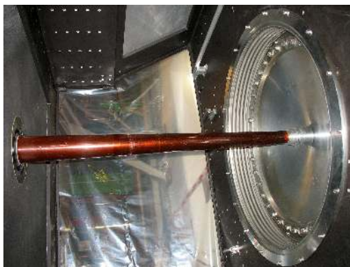
Figure 3.2: View of the VELO exit window and UX85/1 beampipe as installed inside the RICH1 gas enclosure.
