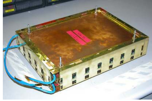
Figure 6.60: GEM chamber fully assembled with the 24 FE electronics boards. The cutouts in the Faraday cage allow the insertion of the cable connectors.
