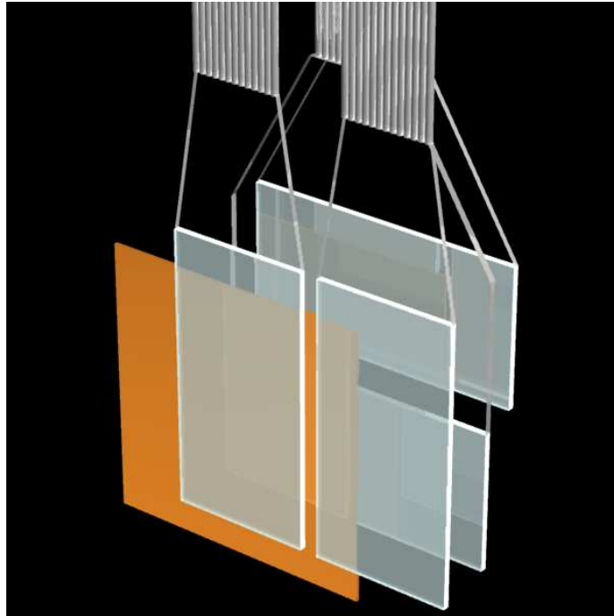
Figure 2.10: A schematic view of a front counter (FC). Two pairs of plastic scintillators segmented in vertical and horizontal directions are indicated by light blue rectangles. A copper plate of 0.5 mm thickness is inserted between the pairs. The scintillator light outputs are fed to PMTs via an acrylic light guide and optical fibers.
