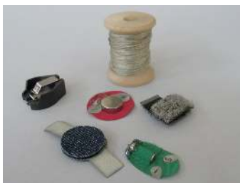
Figure 3. Sensors and actuators, a stitch-able battery holder, and a spool of conductive thread.
