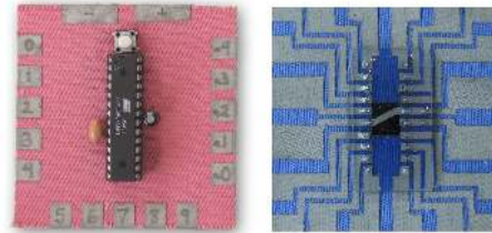
Figure 1. Top and bottom views of microcontroller patches from the first e-textile construction kit.
