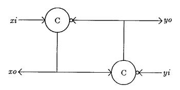
Figure 2: A DI circuit for the one-place buffer
