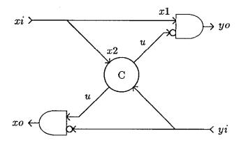
Figure 3: A sequencing element containing isochronic forks
