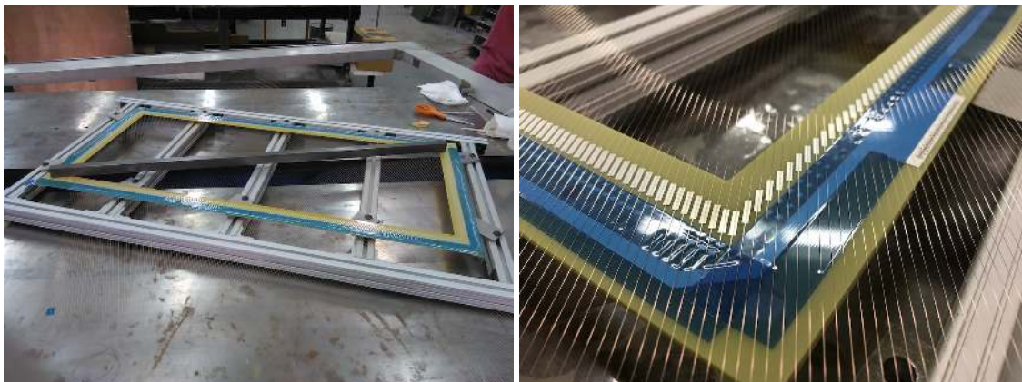
Figure 16. Left: One of the wire planes during transfer, with the wires not yet cut from the winding frame. A steel bar, anchored along the diagonal, ensured that all wires made good contact with the board. Right: Close up view of wires aligned with solder pads prior to attachment with epoxy and solder.
