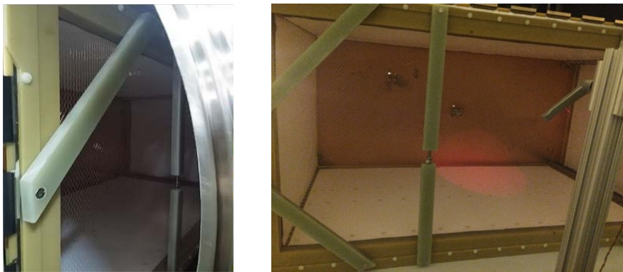
Figure 18. The TPB-coated reflector foils mounted to the TPC’s four field cage walls as viewed through the opening at the front of the inner cryostat ( left ) and looking in from behind the wire planes ( right ).
