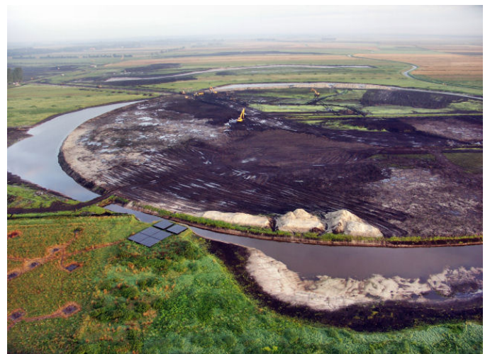
Figure 6: The central area of the LOFAR Core near the village of Exloo in the Netherlands. The inner circle has a diameter of 350 m, the total core area is approximately 2 km in diameter. In the lower left corner, part of a test station is visible. The black rectangles are High Band Antenna tiles. Some Low Band Antennas are only visible from the lack of vegetation around their groundplanes.
