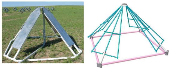
Fig. 3. LWA candidate antennas. Left : “Big blade” design, Right : “Fork” design. Antennas are approximately 1.5 m high. Arms are tilted downward to primarily improve pattern.
