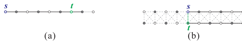
Figure 5. Rectangular supergrid graphs in which there is no Hamiltonian (s, t) -path for (a) R(m, 1) and (b) R(m, 2) , where solid lines indicate the longest path between s and t .
