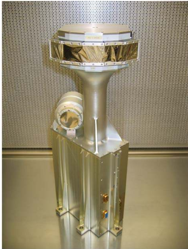
Fig. 3 Photo of the LET and HET and the SEP Central housing. LET is mounted on a post so as to clear the FOV. HET is mounted on top of the SEP Central housing, with its electronics mounted inside. The SEP Central processor and the low-voltage power supply and bias supply for the four SEP sensors are located in this housing
