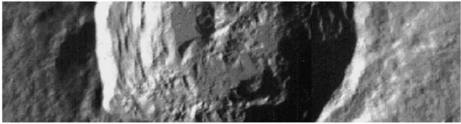
Fig. 6 Clementine LWIR daytime thermal image of Anaxagoras Crater (75°N, 10°W; diameter 52 km) at ~200 m spatial resolution (Lawson et al. 1997), which is similar to the mapping resolution that will be achieved by Diviner
