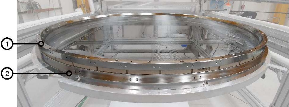
Figure 6: The electron extraction region assembly on the loom. 1-Anode grid; 2-Gate grid. During TPC operations the anode is above the LXe surface and the gate is below. The liquid level is registered to this assembly by three weir spillovers.
