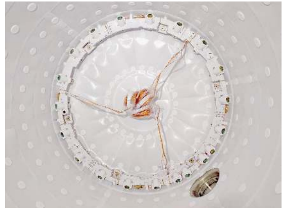
Figure 4: Upper panel: CAD section of the TPC below the cathode showing the location of the 2” bottom side skin (1) and lower dome (2) PMTs. Lower panel: Photograph showing the PTFE panelling attached to the ICV that ensures high reflectance in the skin region and the lower side skin PMT ring at the bottom of the vessel.
