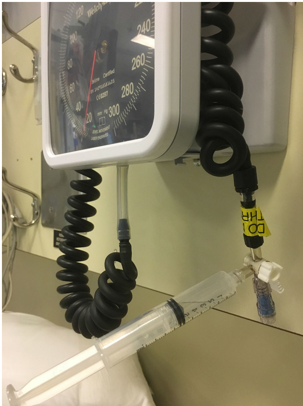
Figure MacGyvered equipment for measuring endotracheal tube cuff pressure fashioned from a three-way stopcock, a 10 mL syringe, and a blood pressure manometer. Given the wide scale of this blood pressure device, and its units in millimeters of mercury and not centimeters of water, accuracy of cuff pressures cannot be guaranteed. Commercial manometers for endotracheal tube cuff pressures are available
