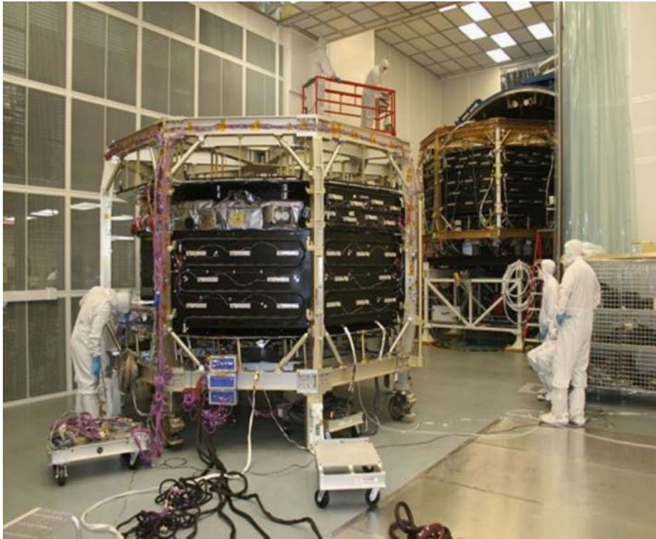
Fig. 44 Observatory #2 being prepared for thermal vacuum testing at NRL
