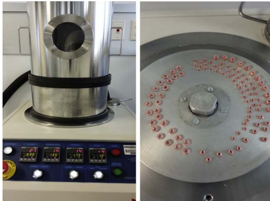
Fig. 3. Parylene coating of copper nuts. Left: the parylene coater. Right: parts on the deposition stand.
