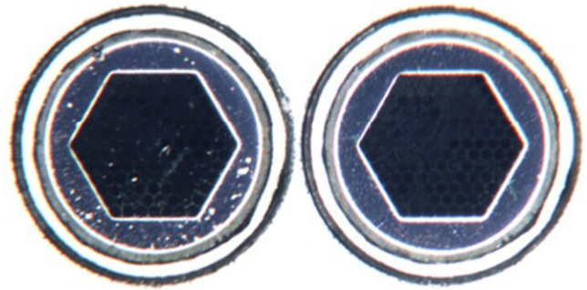
Figure 29. Left: image of 127 fiber IFU Ma.023 with contamination from plugging operations. Aluminum particles can be seen in the center and lower left of the IFU as well as a haze across the lower right caused by finger oil contamination from the plugging operation. Right: the same 127 fiber IFU cleaned with pure methanol.
