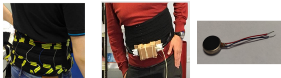
Figure 7. TactiBelt prototype ( left , showing vibrator positions, and center , showing the complete device) and type of used vibrator ( right , RS DC minivibration motor).
