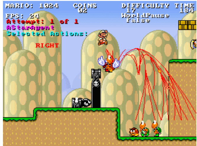
Fig. 4. Visualization of the future paths considered by the Robin Baumgarten’s A* controller. Each red line shows a possible future trajectory for Mario, taking the dynamic nature of the world into account.
