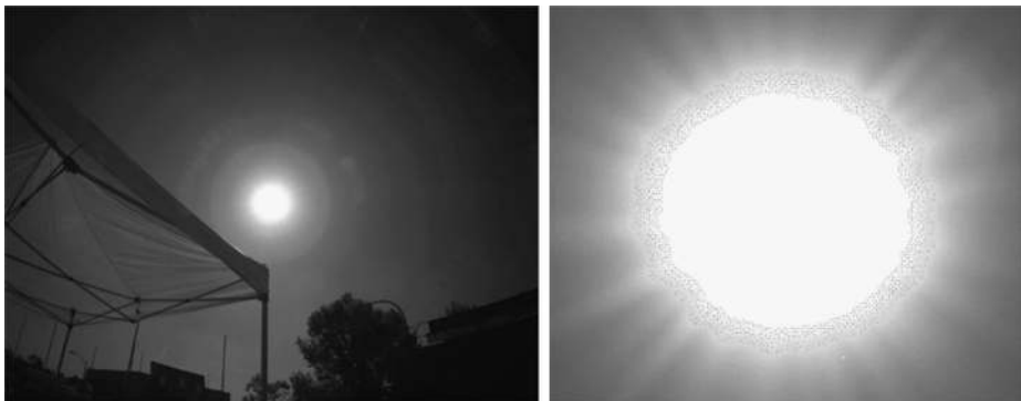
Fig. 34 Examples of Navcam outdoor solar image testing, conducted with a flight-like Navcam. The left image was acquired in quarter-scale ( 4 \times 4 ) mode, and the image on the right was acquired in full-scale ( 1 \times 1 ) mode. The image on the right is cropped to show detail
