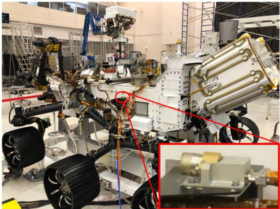
Fig. 27 Location of the EDLCAM microphone on the Perseverance Rover. The microphone is located on the port side (Y-axis, rover coordinate frame) of the rover body, above the middle wheel
