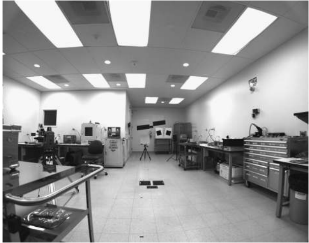
Fig. 40 An MTF test image taken with the LCAM flight unit in the MSSS Cleanroom. This image was acquired unsummed and over the full format of the detector
