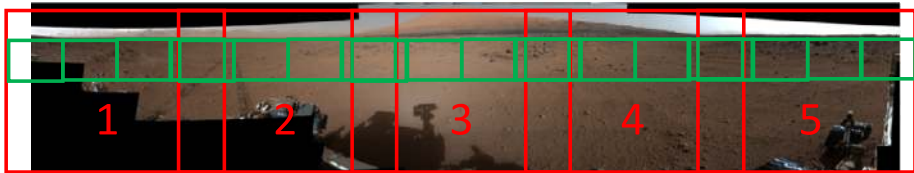
Fig. 43 Notional Navcam 360° survey panorama, comprised of a 5 \times 1 quarter-scale portion (images 1 through 5, shown in red), and a full-scale 360° inset panorama ( 16 \times 1 full-scale tiles, shown in green)
