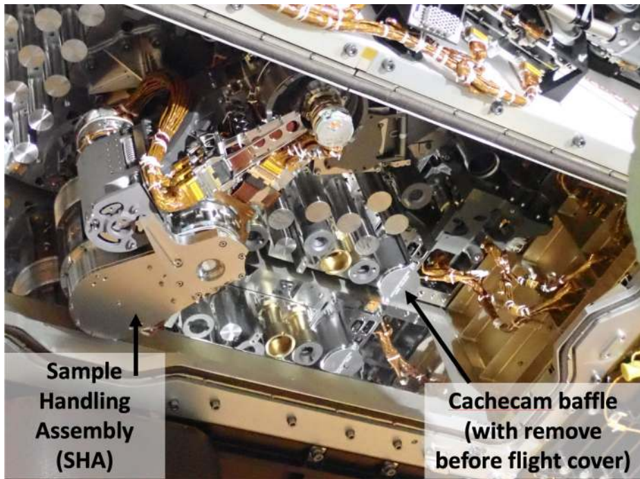
Fig. 20 Location of the Cachecam within the Adaptive Caching Assembly (ACA), looking upwards from below the rover chassis. A portion of the Front Hazcam cover mechanism spring assembly can be seen in the upper right of the image
