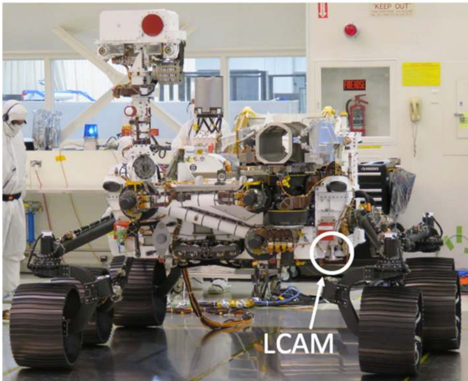
Fig. 30 Location of the LCAM on the rover
