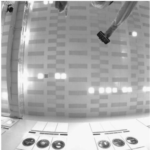
Fig. 41 LCAM image of the ceiling in the JPL Spacecraft Assembly Facility (SAF) taken after integration with the flight rover. This image was acquired in the flight mode ( 2 \times 2 summed with windowing to give a 1024 \times 1024 pixel format)
