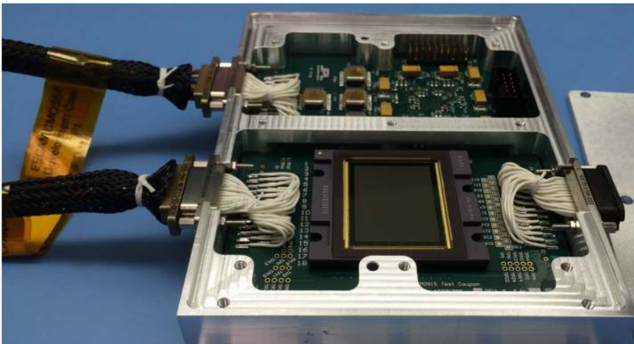
Fig. 11 A CMV-20000 detector undergoing prototype testing in 2014 at JPL. The active imaging area is 32.77 mm × 24.58 mm
