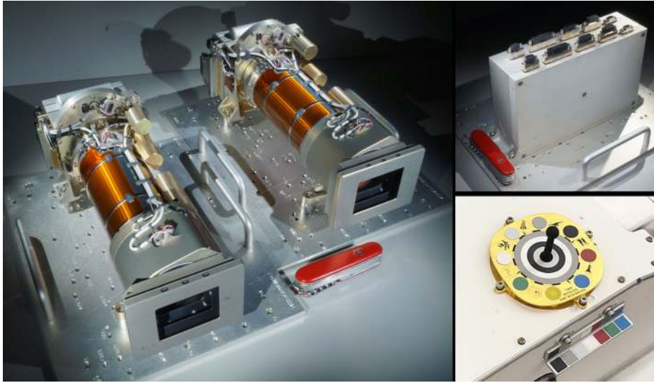
Fig. 4 Mars 2020 Perseverance rover Mastcam-Z flight hardware. (Left) Flight Camera Heads (identical to each other except for different color filters in their filter wheels; Table 3), shown upside-down on temporary carrying plates. (Upper right) Flight Digital Electronics Assembly (DEA), on a temporary carrying plate. For scale, the pocket knife in the photos is 3.5 inches (88.9 mm) long. (Lower right) Flight Primary (top) and Secondary (lower) Calibration Targets, mounted on the rover deck. For scale, the primary target is 3.1 × 3.1 inches (8 × 8 cm) across
