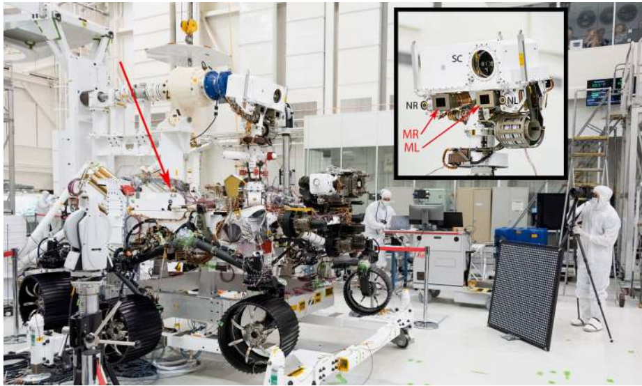
Fig. 8 The Mars 2020 mission's Perseverance rover, in testing at the Jet Propulsion Laboratory in July 2019. The inset shows the top of the rover's Remote Sensing Mast assembly, with the Mastcam-Z left (ML) and right (MR) cameras as well as the rover's two Navcams (NL, NR) and the mast unit of the SuperCam (SC) instrument, including the aperture for the Remote Micro-Imager (RMI) and other SuperCam systems (Maurice et al. 2020; Wiens et al. 2020). The red arrow shows the location of the Mastcam-Z Primary and Secondary calibration targets on the rover deck (see Fig. 4 and Kinch et al. 2020a)
