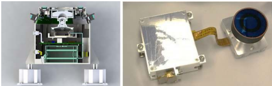
Fig. 36 (Left) Cutaway view of the SkyCam within the RDS. (Right) RDS-SkyCam Flight Model unit
