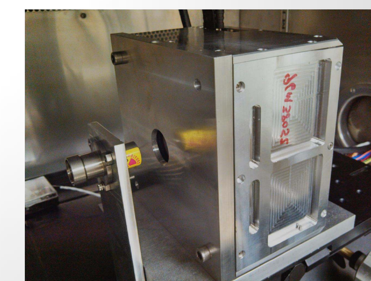
Engineering model of the CLASP camera
