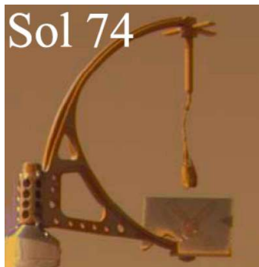
Figure 12. Image of the telltale used to determine estimates of winds at the Phoenix landing site. Adapted from Holstein-Rathlou et al. [2010] with permission.
