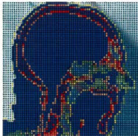
FIGURE 1. CT scan of a head using the fully-specified lattice fill capability of MCNPX.
