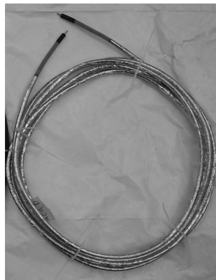
Figure 6: Miniature cable prepared for testing.
