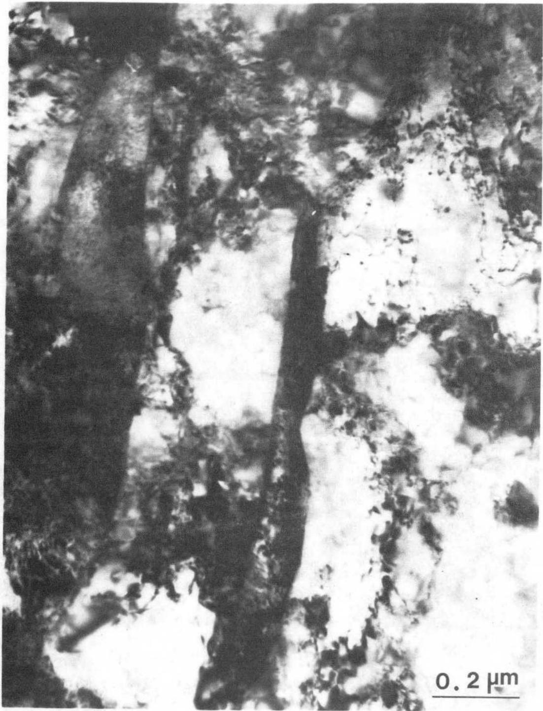
Fig. 6. Bright field TEM micrograph of fresh and tempered martensite in 9 Ni steel tempered 3 hrs at 590°C followed by 25% cold rolling.
