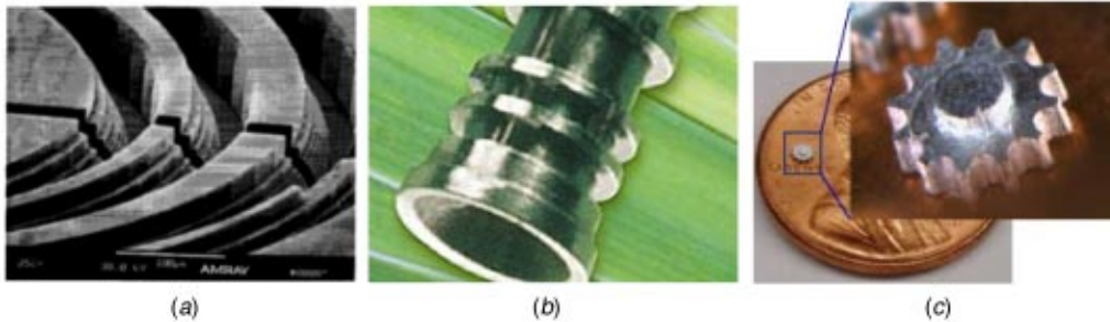
Fig. 1 (a) Micromilled trenches with stepped walls [8], (b) neurovascular device component, and (c) microgear
