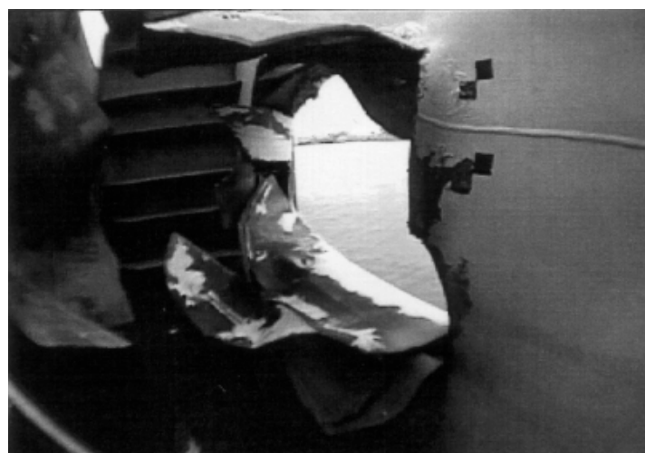
Fig. 3.89. Side damage of full-scale collision experiments sponsored by Japanese ASIS (1998).
