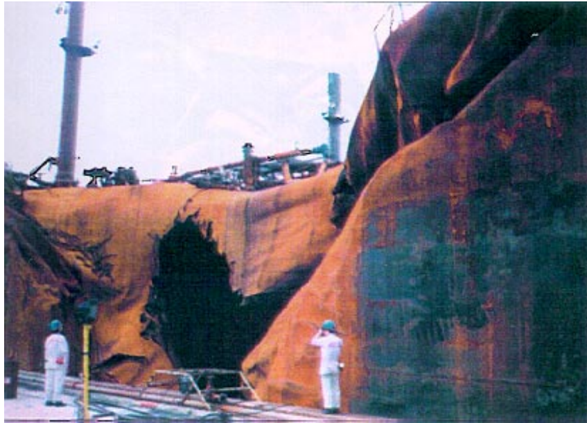
Fig. 1.1. Damage to a 100,000 dwt tanker struck by a 22,600 dwt container ship (1992).
