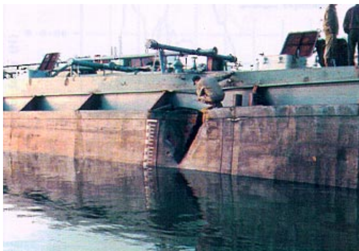
Fig. 3.88. Damage to a ship side struck by a bulb in a collision accident.
