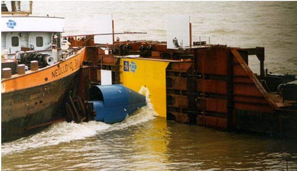
Fig. 3.8. Full-scale collision experiment in 1998 in the Netherlands.
