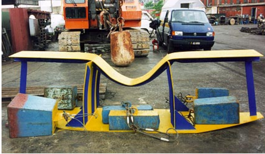
Fig. 3.11. A full-scale side model after collision experiment in Denmark (Qvist et al., 1995).
