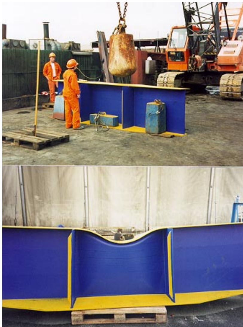
Fig. 3.59. Experiment of a steel ball impacting a side-stringer model (Qvist et al., 1995).
