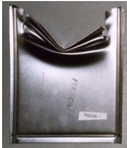
Fig. 3.51. A web model after crushing test (Simonsen et al. 1999).
