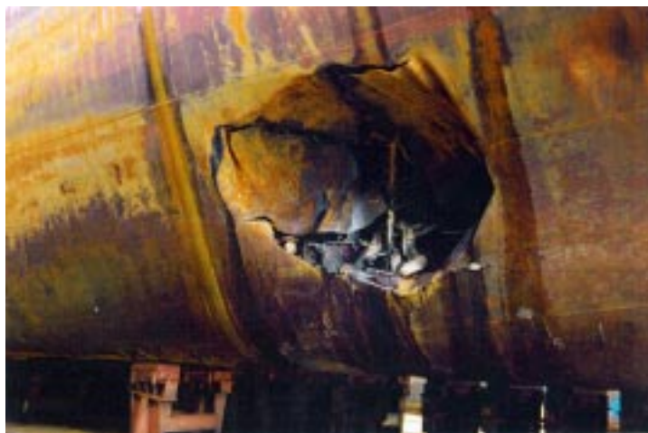
Fig. 3.88. Damage to a ship side struck by a bulb in a collision accident.
