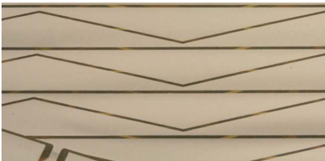
Fig. 24 Double wedge or vernier pads etched on the aluminium deposition of the cathode foil (Color figure online)
