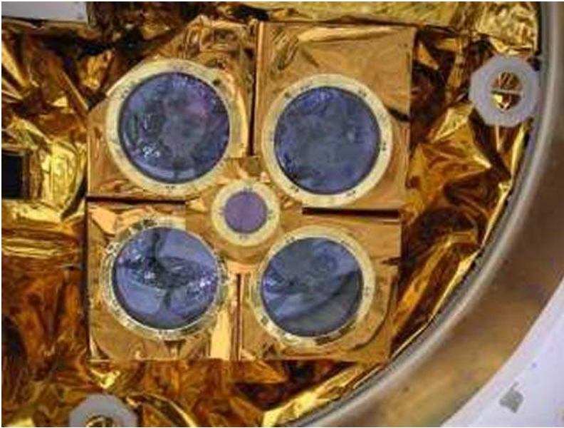
Fig. 18 The MLA instrument shown mounted to the MESSENGER payload deck with thermal blankets installed
