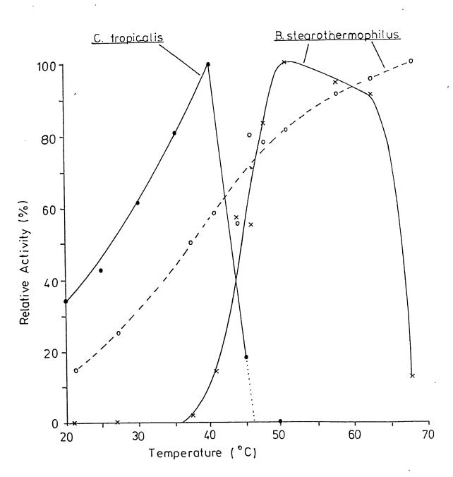
closed circles, CrossesAand solid lines indicate results for phenol hydroxylase. Open circles and dashed line indicates results for the NADH oxidase of <u>B. stearothermophilus</u>.
