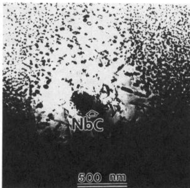
Figure 18. (Nb, Ti)C particle in aged IN625 with \gamma'' denuded around the carbide particle.
