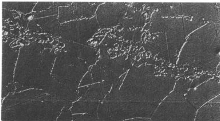
Figure 5. Photograph of Banded Microstructures in A625 Plate (425X)
