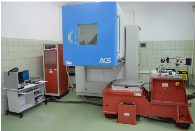
Fig. 1. Test stand for fatigue testing of compressor blades: 1 - climatic chamber, 2 - power amplifier, 3 - computer control system, 4 - electrodynamic vibration exciter
